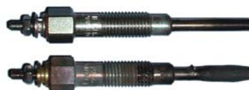
Picture 3. Intact glow plug (above) and damaged glow plug in short circuit (below)
